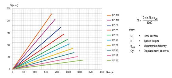
These graphs are the results of testwork done in HYDRO LEDUC R&D laboratory, on a specific test bench with a mineral hydraulic fluid ISO VG46 at  $25^{\circ}$ C (~100 cSt) - disregarding the volumetric efficiency.
