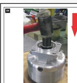
Hit the shaft with a plastic hammer until the shaft comes off from the bottom.
