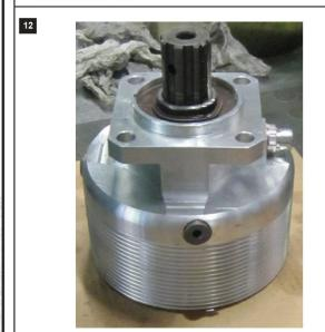
Place both bushing and oil seal on the shaft. Slightly hammer them alternative (make sure they don't separate in this phase) until they are properly in their seat.
