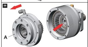
Extract the whole FRONT BODY (position A). Check the integrity of the bearing (see page 15, position 18) placed at the bottom of the REAR BODY.
