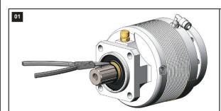
Remove the Seeger ring on the output shaft ensuring not to damage it.
