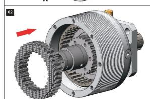
Insert the disks paying attention to ensure the proper alignment between external and internal teeth.
