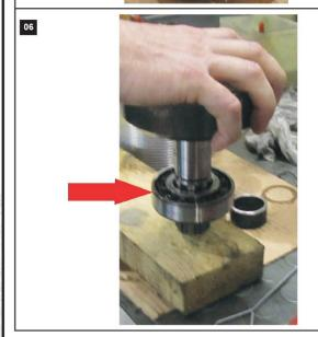
In order not to damage the shaft, place it on a wooden surface and hit the shaft onto it until the bearing slips off. Replace the bearing.
