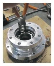
Take the other half SLICK SHIFT body, separated at point 01. Remove the Seeger ring (see page 15, position 29) from the hub and then the complete Hub Unit. Extract also the axial bearing and replace it.
