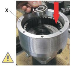
**ATTENTION!** Check that "reaction disk" indicated with "**X**" has remained in its original position, if not re-place it properly with the right orientation.
