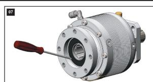
Remove the oil seal by means of a screwdriver. The oil seal must be replaced with a brand new one.
