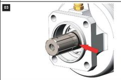
The one indicated in the picture is a static gasket placed under the bushing.
