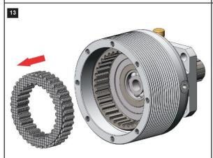
Extract all the disks and check them CAREFULLY. In case they are even slightly damaged or worn out they must be replaced.
