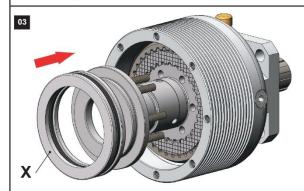
Place springs, "pressure disk" and axial bearing **X** in their housing.
