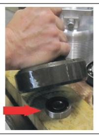
Hit the opposite side of the shaft on the wooden surface until the internal bearing comes off. Replace it.
