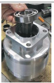
Rotate the Slick Shift and place the new bearing in its seating.
