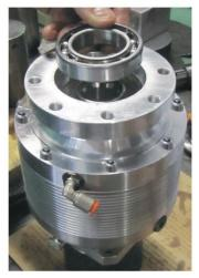
Place the new bearing and, in sequence, the Seeger ring on the hub and a new oil seal. **Seal Kit code 10399030053.**
