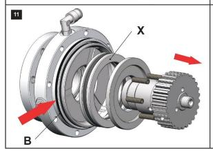
Extract the HUB UNIT including springs, "pressure disk" and axial bearing **X**.
