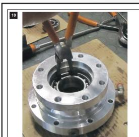
Rotate 180° the body, remove the Seeger ring which is "holding" the bearing.
