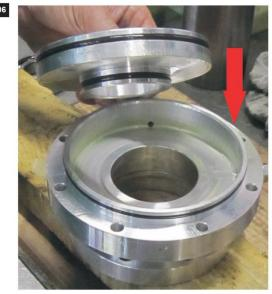
On the other half Slick Shift body, insert indicated piston as shown.
