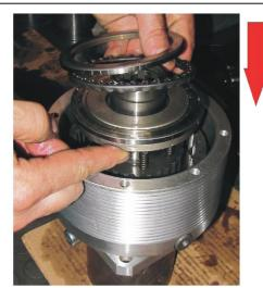
Insert in sequence the "pressure disk" (check correct mounting side) and the new axial bearing.
