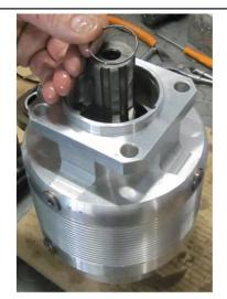
Place the new O-Ring on the shaft.
