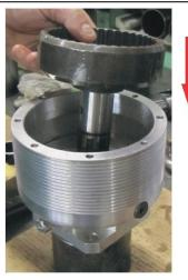
Place the shaft and then the new bearing on the bottom.
