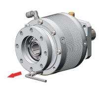
Unscrew all the 8 TCE M8x40 screws by means of an Allen Key.
