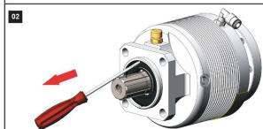
Remove elastic ring and oil seal.
