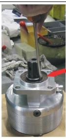
Remove the oil seal by means of a screwdriver. The oil seal must be replaced with a brand new one.
