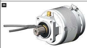
Place again the Seeger Ring. In case it got damaged it must be replaced!
