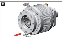
Unscrew all the 8 TCE M8x40 screws by means of an Allen Key.
