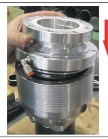
Couple the half body indicated in step n.6 with the other half body assembled before. Screw in the 8 screws with tightening torque = 25 Nm.
