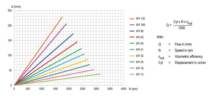
These graphs are the results of testwork done in HYDRO LEDUC R&D laboratory, on a specific test bench with a mineral hydraulic fluid ISO VG46 at 25°C (~100 cSt) - disregarding the volumetric efficiency.
