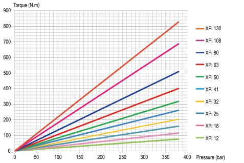
$$C = \frac{\text{Cyl x } \Delta P}{62.8 \text{ x } \eta_{\text{meca}}}$$
