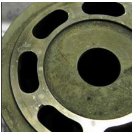
Cylinder barrel with severe damaged surface at the porting. The damage depends on contaminated oil due to poor filtration, clogged filter, previous break down or bad handling when filling the reservoir.
