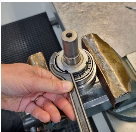
14. Untighten the round nut and remove locker rings.
