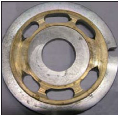
Valve plate with scratched surface.
