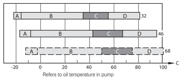
E.g. Hydraulic oil 32: The designation "32" denotes the viscosity is 32 cSt at 40 °C. Lowest start temperature is -23 °C and highest working temperature 82 °C. Ideal working temperature is 35 - 55 °C.
