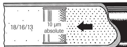
Max 64,000 particles > 5  $\mu\text{m}$ /100 ml.
