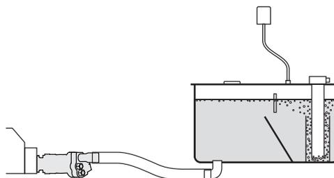
The pump can be installed in 4 positions with the angle upwards, downwards or to the side. When the angle is to the side it is an advantage if the pump can be twisted so that the suction connection is highest.
