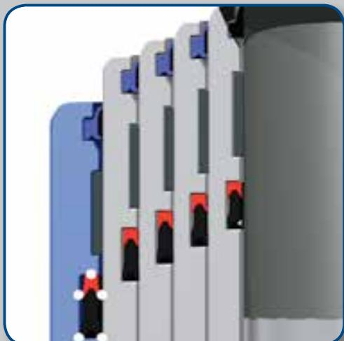
*Double lip wiper seal ensures efficient lubrication of each tube and prevents contamination of the cylinder.*
