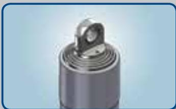
This variant of eye type will ensure that there is no bending stress imposed on the body and reduces cylinder side loading but it will allow more body movement under sideload conditions.
