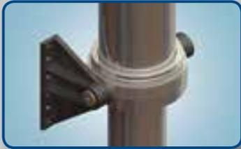
The outer cover design is very strong and suits simple square fronted body designs. Stroke variants do not affect mounting centres but the cylinder reduces the available body length because a cab gap is required. The extra strength has a weight penalty but it may facilitate a simple and light body design.
