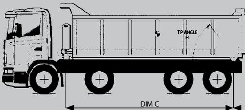
$$\text{Approx stroke} = \text{Tip angle (H)} \times \text{Pivot length (Dim C)} / 59$$
